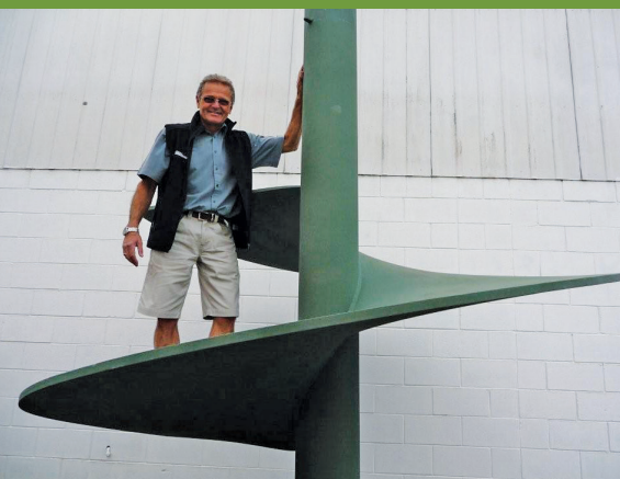
2.4m diameter x 1.2m pitch x 25mm thick drill auger flight
