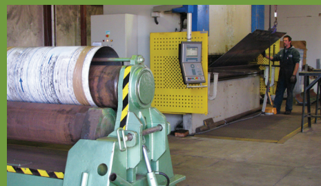
3 metre pinch rollers with 400 tonne, press brake in background
